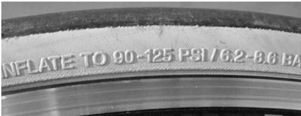
See the sidewalls of the tyre for the manufacturer's Pressure guidelines (Pound per Square Inch -PSI .
